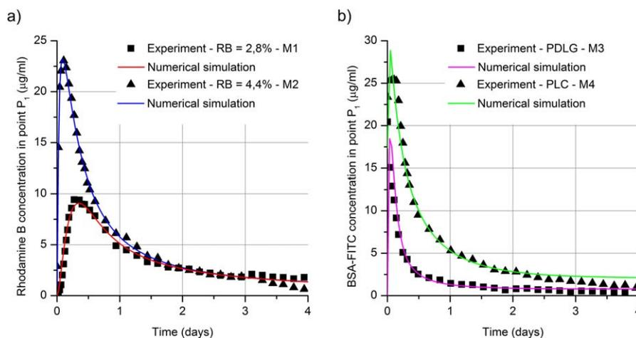
**FIGURE 8.** Real-time concentration profile of a) Rhodamine B, b) BSA-FITC in the point  $P_1$  vs. time (only every tenth point presented for readability). Points represent experimental data. Lines represents results from numerical simulations with parameters of mathematical model  $k_{ads}$ ,  $k_{des}$  fitted. [Color figure can be viewed in the online issue, which is available at [wileyonlinelibrary.com](http://wileyonlinelibrary.com).]
