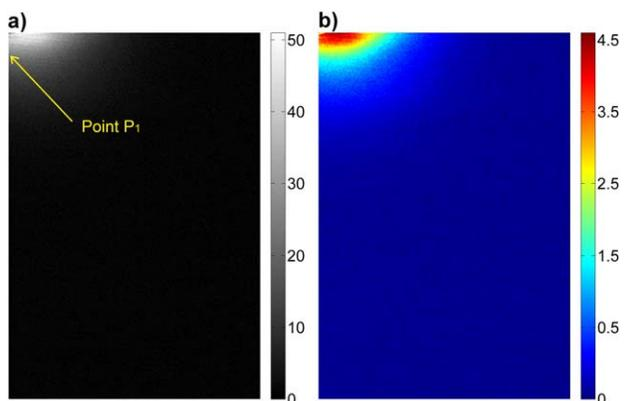
**FIGURE 6.** a) Rhodamine B intensity and b) calculated Rhodamine B concentration in the cuvette. Pictures present one half of the cuvette (left edge—axis of symmetry). [Color figure can be viewed in the online issue, which is available at [wileyonlinelibrary.com](http://wileyonlinelibrary.com).]
