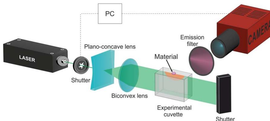
**FIGURE 1.** Experimental setup for drug release evaluation. From left to right: laser with excitation wavelength suitable for examined model drug, round shutter connected with PC, light sheet setup, nanofibrous material in experimental cuvette, emission filter suitable to pass wavelength corresponding to emission of examined model drug, camera connected with PC. [Color figure can be viewed in the online issue, which is available at [wileyonlinelibrary.com](http://wileyonlinelibrary.com).]
