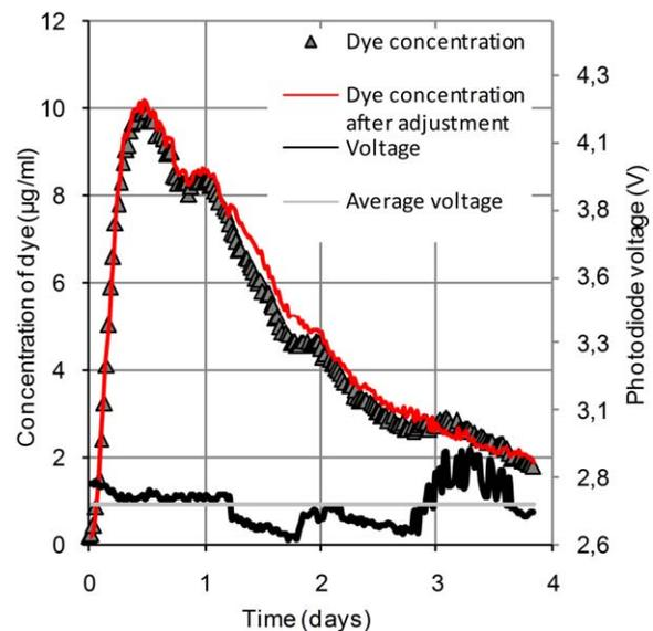
**FIGURE 7.** Concentration of Rhodamine B (gray triangles) in point  $P_1$  and measured photodiode voltage corresponding to laser power fluctuations. Red line presents concentration adjusted to voltage fluctuations. Horizontal gray line represents average value of measured voltage. [Color figure can be viewed in the online issue, which is available at [wileyonlinelibrary.com](http://wileyonlinelibrary.com).]
