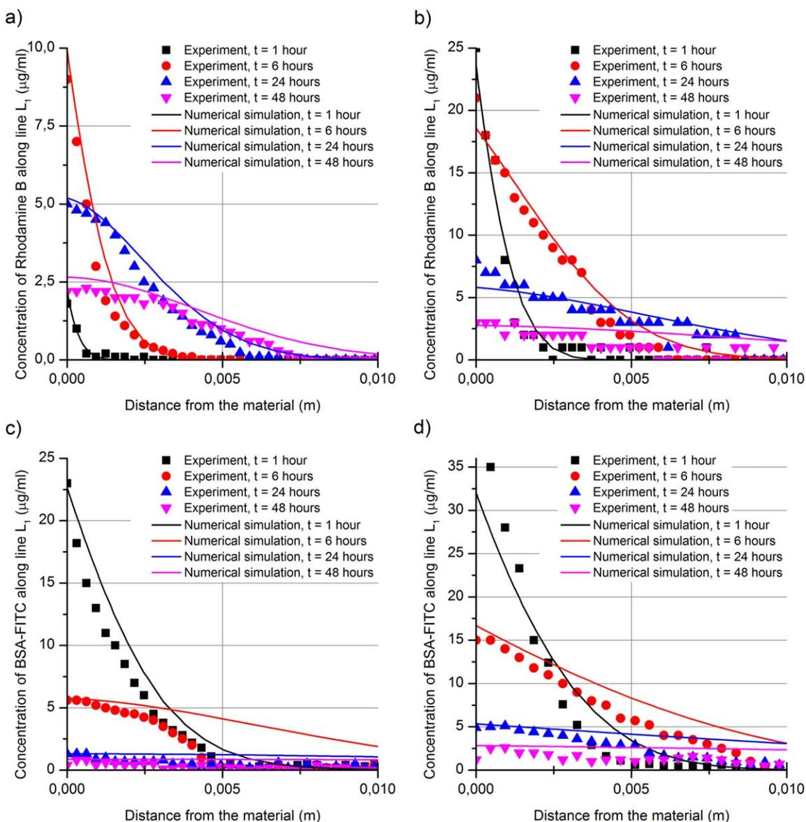
**FIGURE 10.** Dye concentration in hydrogel in the function of distance from the materials for different times of the experiment: 1 h, 6 h, 1 day, and 2 days. Materials containing Rhodamine B: a) M1, b) M2 and BSA-FITC: c) M3, d) M4. Points represent experimental data, lines represent numerical simulations. [Color figure can be viewed in the online issue, which is available at [wileyonlinelibrary.com](http://wileyonlinelibrary.com).]
