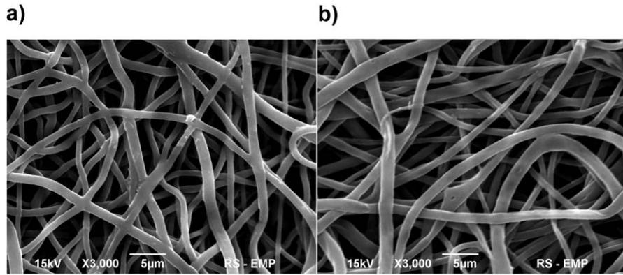
**FIGURE 5.** Morphology examination from SEM micrographs of two materials removed from the hydrogel after 4 days of drug release experiment. SEM micrographs present materials made from two polymers: a) PDLG polymer—M3, b) PLC polymer—M4.
