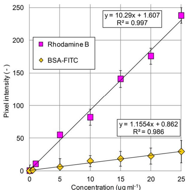
**FIGURE 2.** Calibration curves of Rhodamine B and BSA-FITC in PVA hydrogel. [Color figure can be viewed in the online issue, which is available at [wileyonlinelibrary.com](http://wileyonlinelibrary.com).]
