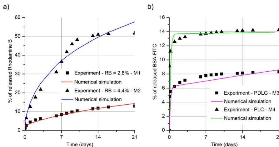
**FIGURE 9.** Release profile from materials with two different initial concentration for Rhodamine B a) BSA-FITC b). Drug release experiment was conducted with standard methods in vials filled with buffer. Points represent experimental data. Lines represent results from numerical simulations with parameters of mathematical model  $k_{ads}$ ,  $k_{des}$  fitted. [Color figure can be viewed in the online issue, which is available at [wileyonlinelibrary.com](http://wileyonlinelibrary.com).]
