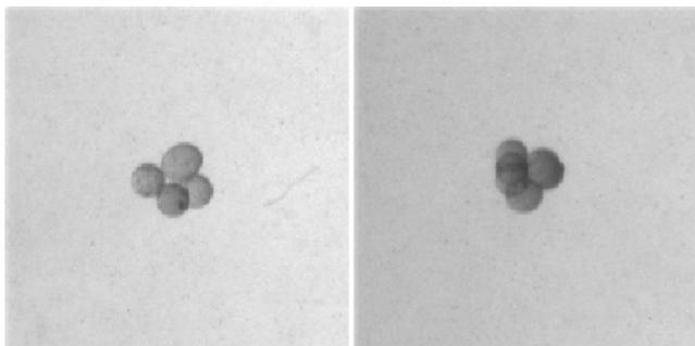
FIG. 2. Clusters with a small even number of particles at an almost symmetric configuration translated as a rigid body (Experiment Nos. 34 and 43 in Table I).
