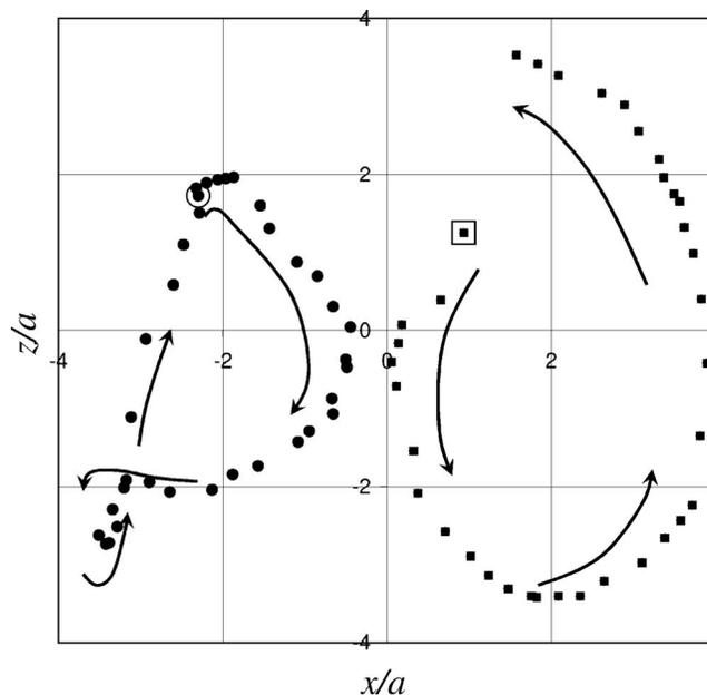
FIG. 6. Exemplary trajectories  $[x(t), z(t)]$  of two particles from a cluster which consisted of 14 particles (Experiment No. 31, see Table I). Positions of the particles are plotted relatively to the center of the cluster and scaled by the particle radius  $a$ . The initial positions are circumscribed with a square and a circle.
