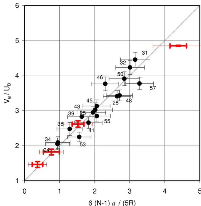
FIG. 9. (Color online) Correlation of the measured cluster settling velocities  $V_e/U_0$  with the ensemble-averaged velocities  $6(N-1)a/(5R)$  of point-particle clusters: dots—present results, crosses (red)—experimental and numerical results from Refs. 9 and 10 (superimposed), and straight line—Eq. (1).
