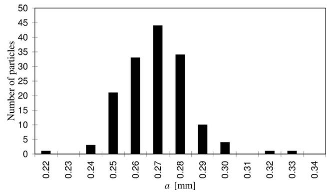
FIG. 1. Distribution of radii of the particles in all the clusters investigated experimentally (measured from the images).
