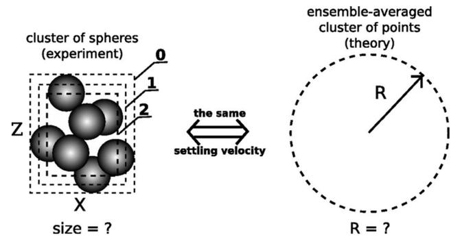
FIG. 8. To apply the point-particle model to the experiment, three effective radii  $R$  were tested for three values of  $\xi$ , depicted as frames 0, 1, and 2.
